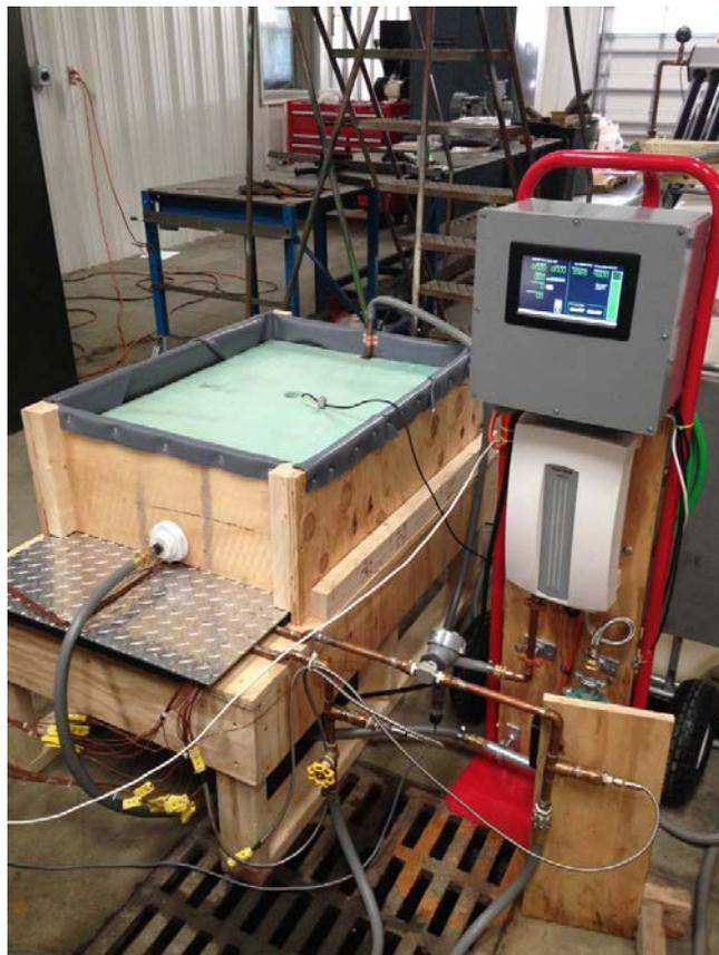
*Figure 3 – Purdue hog cooling pad testing apparatus.*
