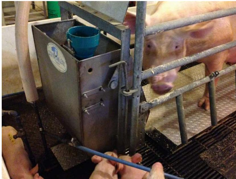
*Figure 4 – Purdue prototype hog cooling pad being tested in farrowing house.*
