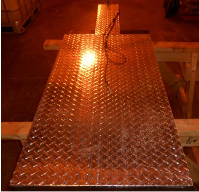
*Figure 2 – Current prototype of Purdue hog-cooling pad.*
