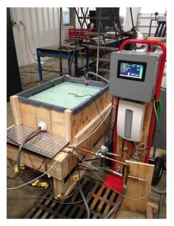
*Figure 3 – Purdue hog cooling pad testing apparatus.*
